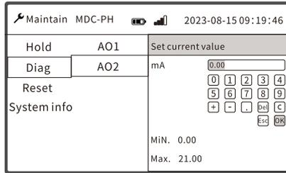
Fig.57 Output current setting
