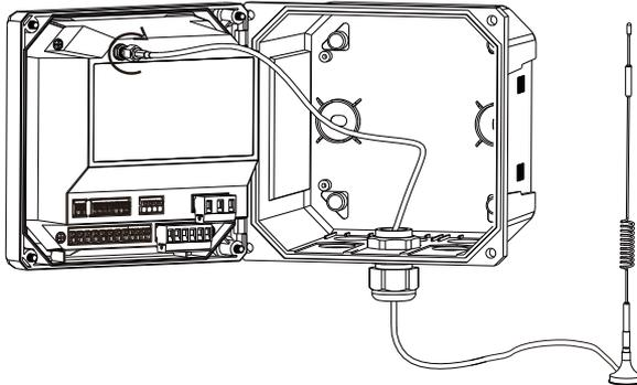
Fig.16 Wireless communication wiring schematic
