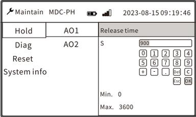
Fig.51 Setting the hold release time
