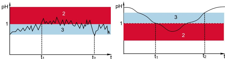
The graph on the left shows the hysteresis effect for a high alarm, while the one on the right illustrates the hysteresis effect for a low alarm.
