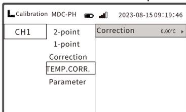
Fig.48 Temperature correction
