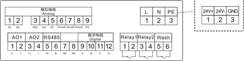
Fig.8 Terminal definitions (single channel)
