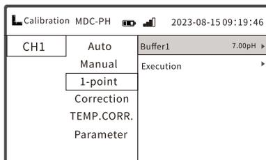
Fig.41 1-point calibration
