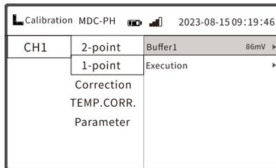
Fig.46 1-point calibration
